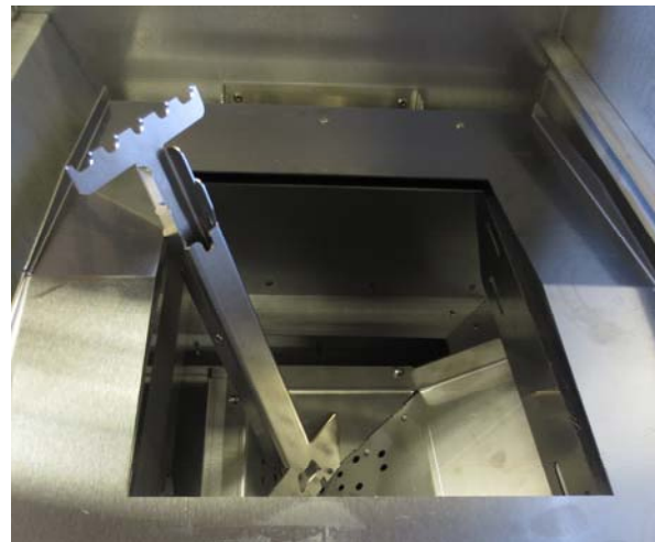
Step 3: Cleaning of the Burn Pot
