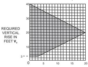
HORIZONTAL VENT RUN PLUS OFFSET IN FEET H, The shaded area within the lines represents acceptable values for H<sub>+</sub> and V<sub>+</sub>
