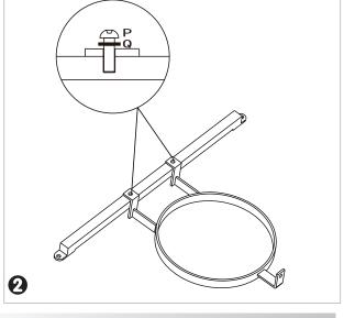
3 Turn the assembled panels upside-down, then attach Tank Support Bar ● to Panels ④/ by aligning holes at each end of Tank Support Bar with holes at the bottom of Panels. Insert Bolt through Washer into holes. Tighten gently with Hex Wrench . Then attach Tank Support Ring ● to the Leg of Door Panel ● by aligning hole in front of Tank Support Ring with hole in Leg. Insert Bolt ● through Washer ● and then into the hole. Tighten with Hex Wrench ●.
