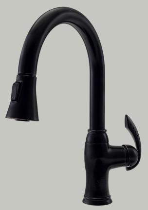
2 1/4" x 9 1/4" x 14 5/8" 1- or 3-Hole Installation Ceramic Disc Cartridge 56" Flexible Metal Hose Completely Pressure Tested ADA Approved Constructed of Lead-Free Materials Complies with NSF Standards **SDWA Compliant** cUPC Certified (Uniform Plumbing Code) Lifetime Warranty Antique Bronze Finish
