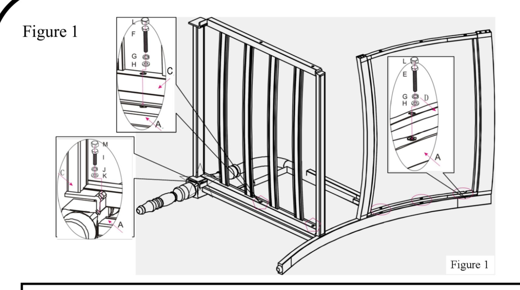
Repeat the steps in figure 1 to assemble the right arm (B). Once all pieces are assembled and tighten all bolts with wrench (N), and cover using bolt covers (L) and large bolt covers (M).
