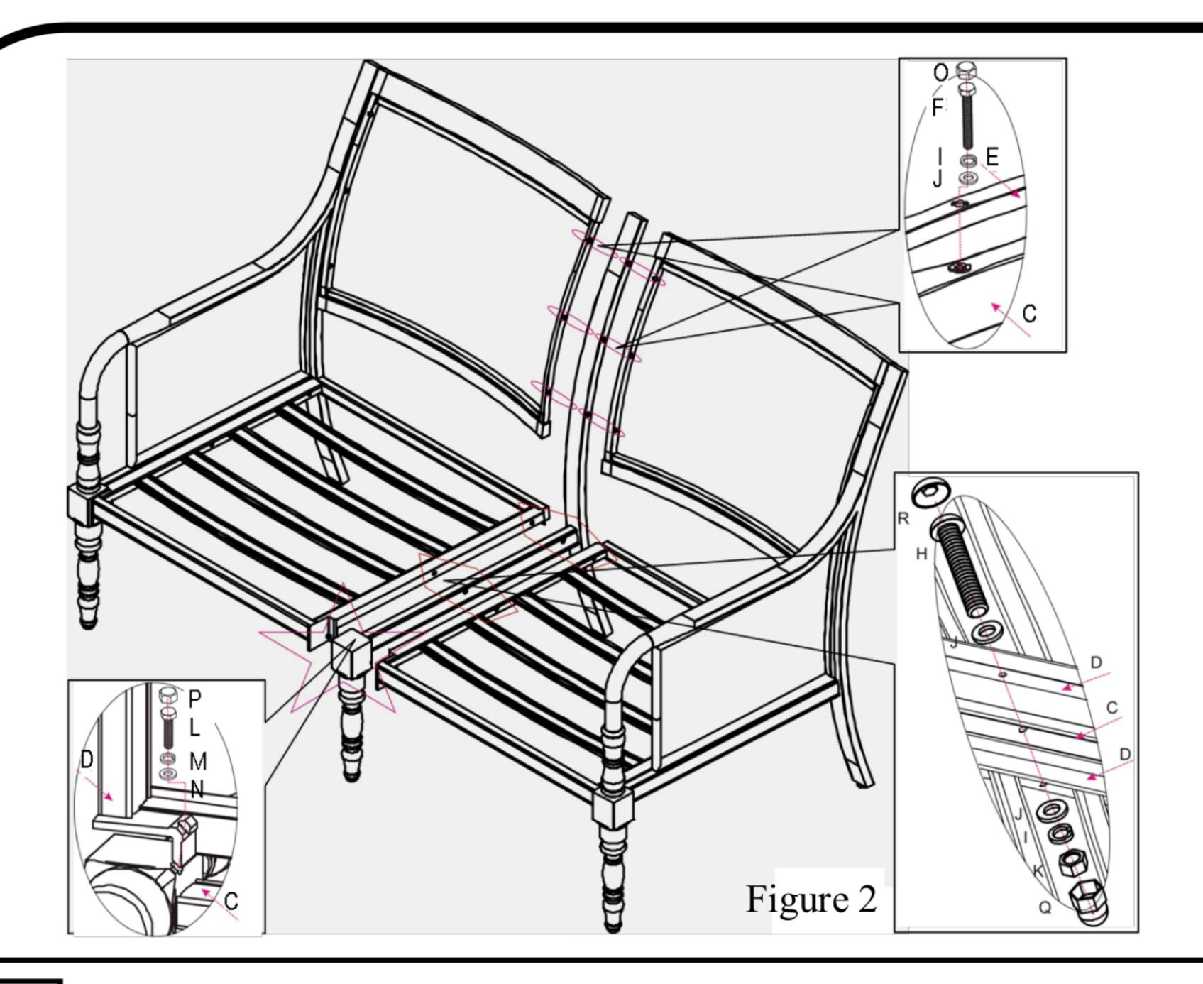
Once all pieces are assembled hand tighten all bolts, and cover using nut covers (Q) and bolt covers (R).
