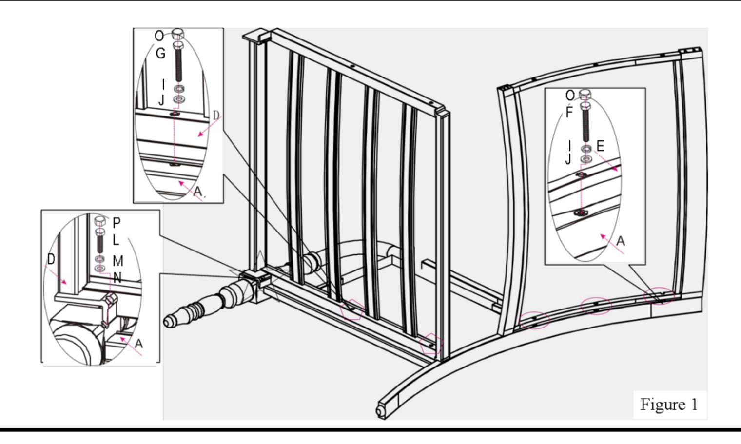
Repeat the steps in figure 1 to assemble the right arm (B), back (E) and seat (D) assembly.
