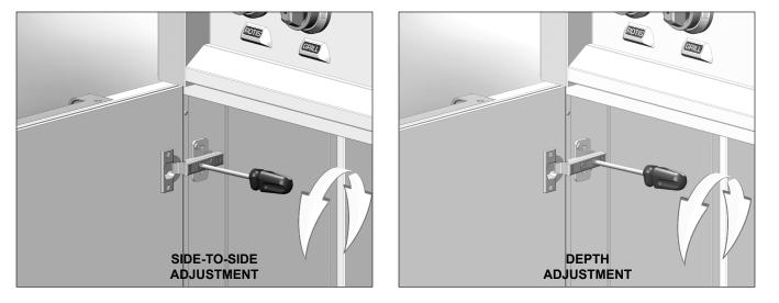
18. The side and depth adjustment of the doors are shown below.
