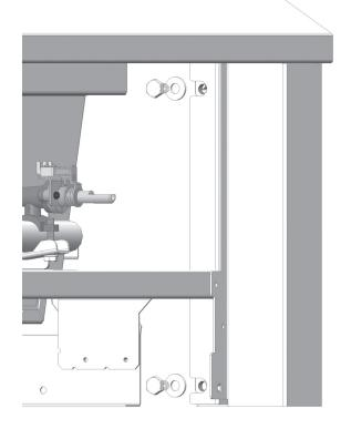
12. Install 1 flat washer and hex bolt at the rear inside wall of the cart as shown here using a 7/16" wrench or socket wrench. Repeat this on the opposite side of the cart. If all cart panels are properly aligned with the grill head, you may now tighten all the bolts.
