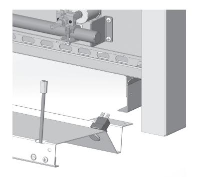
11. Reach inside the right front area of the cart wall and install 2 flat washers and hex bolts as shown here using a 7/16" wrench or socket wrench. Do not tighten yet. Repeat this on the opposite side of the cart.
