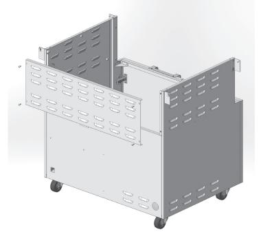
3. Open the right door and install the electrical box supplied with your grill on the 2 studs at the rear, inside wall of the cart. Pass the electrical cord through the square hole. Reinstall both nuts and tighten with 3/8" wrench or socket wrench.
