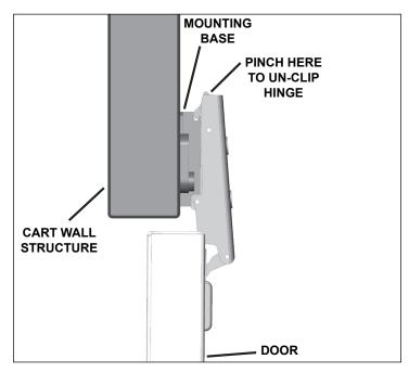
17. Aspire doors feature 3-way adjustable hinges. It is recommended to do the height adjustment first. Loosen the top & bottom screw on each mounting base, then use the height adjustment screw shown below to fine-tune the vertical height of the door in the cart. Tighten the top and bottom screws when done.
