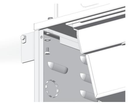
**Note:** If the holes do not wish to align, a large bar-clamp may be used as shown below to help pull everything together. Use rags or small pieces of cardboard to cushion the clamp and not scratch the finish on your grill and cart.
