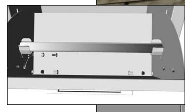
1. Locate the Two Hinge Screws & the Single Pin Screw and remove all Three to remove Towel Holder.
