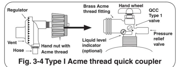
Fig. 3-4 Type I Acme thread quick coupler
