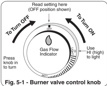
Fig. 5-1 - Burner valve control knob
