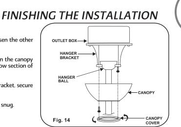
Step 1. Remove 1 of the 2 screws from the bottom of the hanger bracket and loosen the other one half a turn from the screw head.
