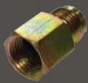
U3-6C-S Steel Gas Flare Fitting, 3/8" OD Flare x 3/8" FIP
