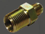
U1-6D-S Steel Gas Flare Fitting, 3/8" OD Flare x 1/2" MIP (Tapped 3/8" FIP)
