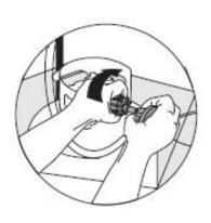
the unit to the "HIGH" position for about 20 seconds to allow the air in the system to purge before attempting to light the burners.
