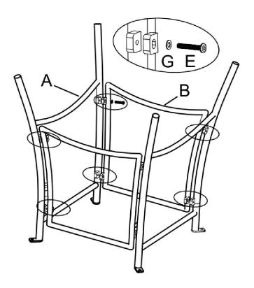
Attach the Legs to the Table Top at the connection points on the supporting bars using Washers(G) and Bolts(F) with Allen Key(H) as Figure 2.
