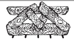
Important: Adequate ventilation is absolutely necessary. Adequate spacing between the logs is NECESSARY and MUST be maintained. Some carbon build up (sooting) may occur where flames strike the logs. If carbon build up (sooting) continues, rearrange top logs to allow more opening(s) for flame(s) before sooting becomes worse. If any sooting occurs outside of the firebox (i.e. on the walls), turn off unit immediately and contact a qualified professional service technician.
