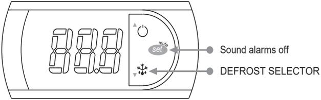
If the cabinet temperature is displayed, the cooler is working properly; if an alarm code is displayed, see the information below
