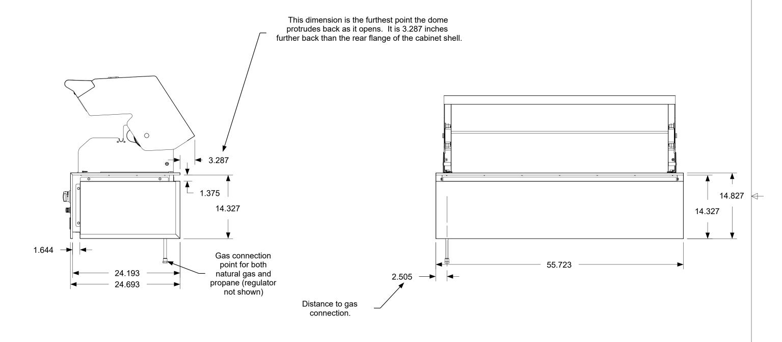
The dimensions shown are the actual physical dimensions of the grill. Additional clearances to cabinetry are dependent on the tolerances of the cut-out. The suggested cut-out dimensions are listed in the chart below but these dimensions can be reduced if the tolerances are controlled.
