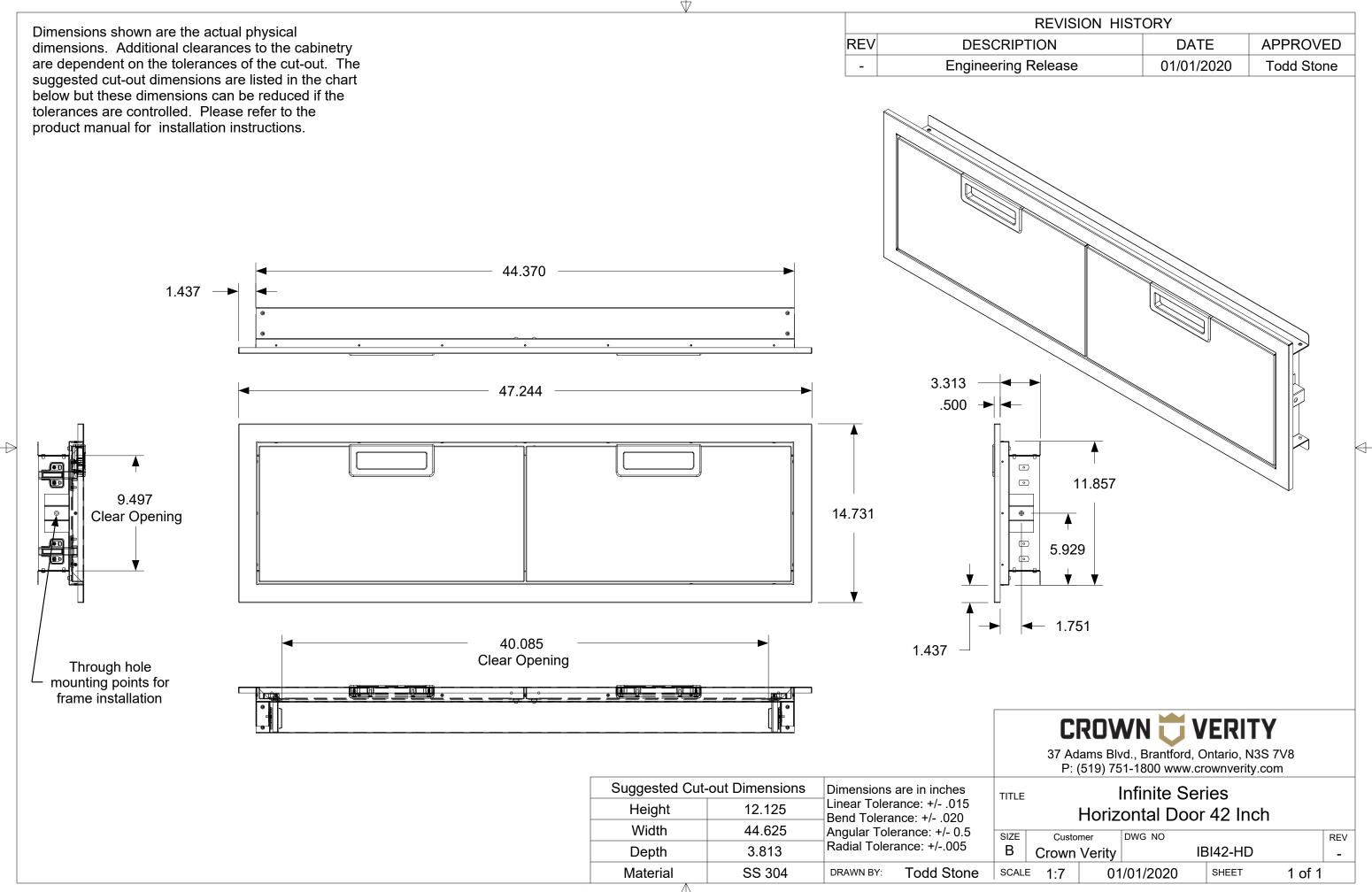
Dimensions shown are the actual physical dimensions. Additional clearances to the cabinetry are dependent on the tolerances of the cut-out. The suggested cut-out dimensions are listed in the chart below but these dimensions can be reduced if the tolerances are controlled. Please refer to the product manual for installation instructions.
