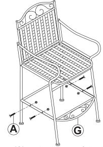
• Secure Footrest (G) to the bottom of the leg panels using four M6x40mm Bolt Sets (A).
