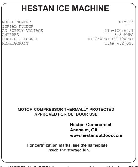
Note: In the "MODEL NUMBER" the \_ references either a (L) Left or (R) Right hinge model
