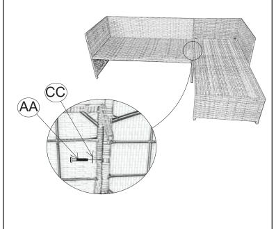
Do not fully tighten hardware until all components in this step have been connected.
