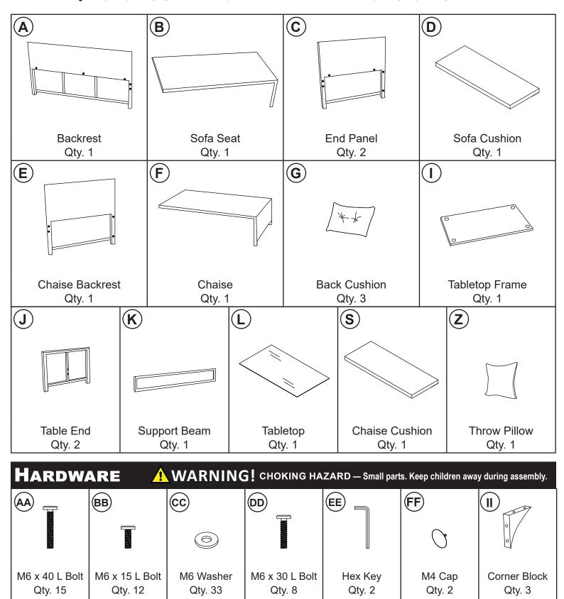
**! HELPFUL HINT:** Do not tighten hardware until all components have been loosely assembled. If the hardware is tightened too soon, mounting holes may not align, and parts may not easily fit together.
