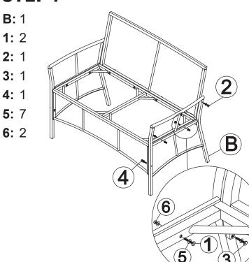
Do not fully tighten hardware until all components in this step have been connected.
