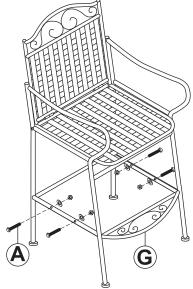
• Secure Footrest (G) to the bottom of the leg panels using four M6x40mm Bolt Sets (A).
