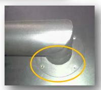
Attach the Smoke Stack (1) to barrel end by first installing the second Felt Gasket (2) between the Smoker Stack (1) and the barrel end. Then, using the four (4) screws, previously removed from the barrel end, secure firmly to the barrel end. Once this is complete, tighten the other four loosely mounted screws on the cabinet end, to finish securing the smoke stack on both ends.
