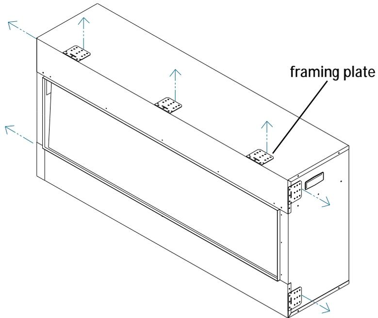
3. Re-fix the framing plates to the unit as the picture shows
