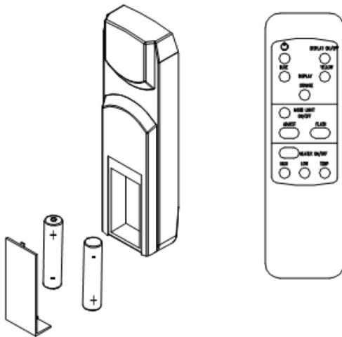
For remote to function make sure the heater is plugged in and main power switch located on the bottom left hand side is at position I.
