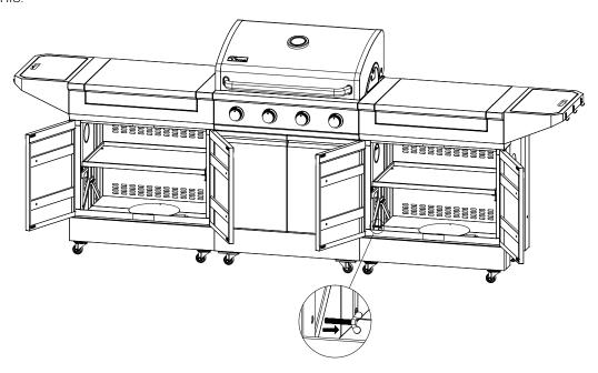
5. To connect a gas tabletop to the **RIGHT** Grill & Prep Cart, remove the center prep table.
