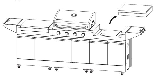
**9.** Place the tabletop unit into the chassis.
