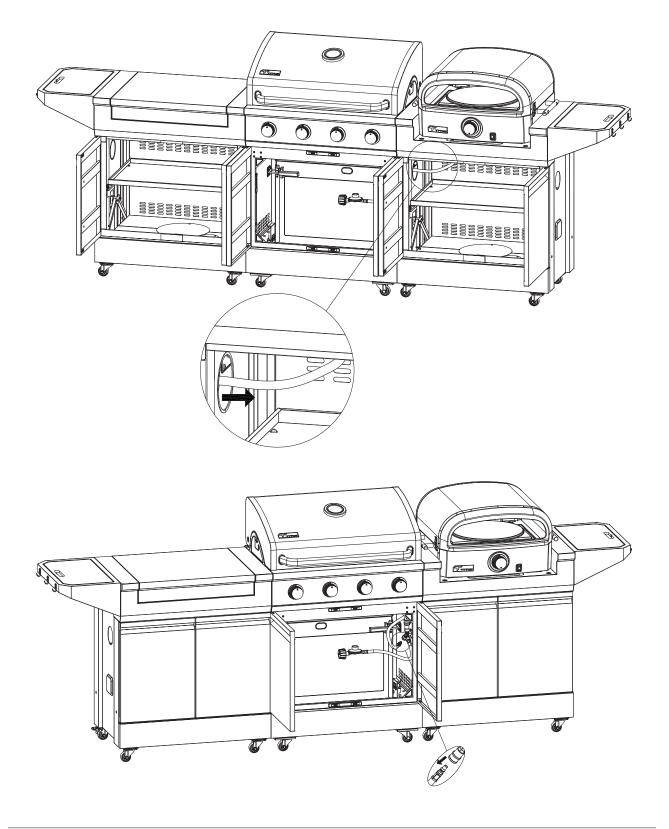
**8.** To connect an electric or charcoal tabletop to the left or right Grill & Prep Cart, remove the center prep table.
