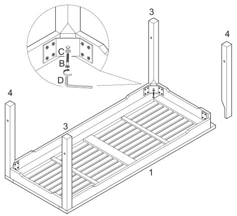
Carefully lay table top (1) upside down on a soft surface. Slide legs (3,4) into place and secure to table top (1) using bolts (B) and washers (C). Tighten bolts (B) with wrench (D).
