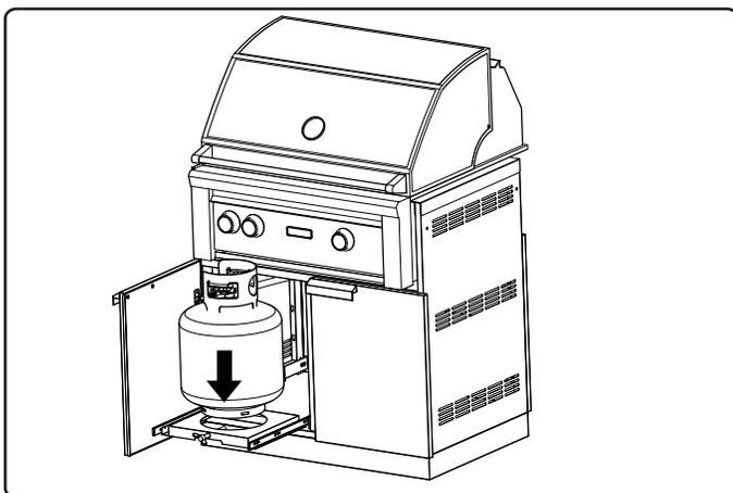
**5** Turn Wing nut bolt until it is seated in tank slot at bottom of tank.
