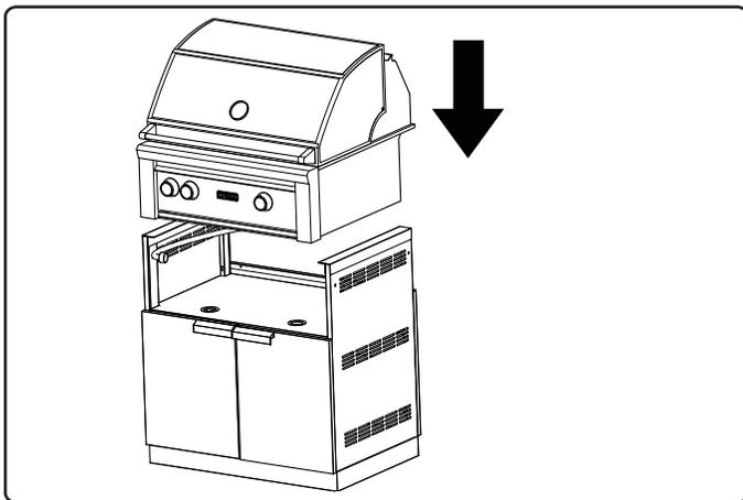
**3** Once the BBQ is centered on the Cart lift up edges of BBQ and Dab a little silicone on the rails to hold it in place
