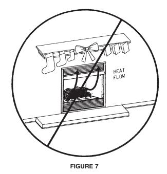
No greeting card, stockings, or ornamentation of any type should be placed on or attached to the fireplace. This is a heating appliance. The flow of heat can ignite combustibles.
