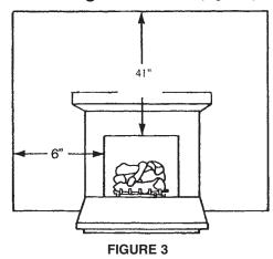
The sides of the fireplace opening must be 6" from any combustible wall. The ceiling must be at least 41" from the fireplace opening.
