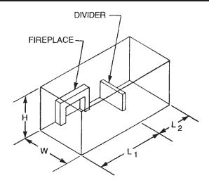
The following formula can be used to determine the maximum heater rating per the definition of unconfined space:
