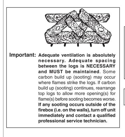
WARNING: Use ONLY Real Fyre burners and valves with this Real Fyre gas log set. Failure to do so may result in property damage or personal injury, and will void listings, certifications, and invalidate claims made to RHP. Contact your local Real Fyre dealer if you need more information.
