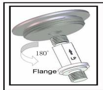
Step 3: Turn the Stem 180°so that the Flange is at The Bottom.
