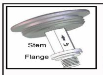
Step 4: Screw the Stem back into the Cap and then reinstall the Cap/Stem Assembly back into the Regulator.
