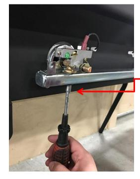
Undo the bolts screw on the bottom of the valve connecting it to the manifold. The manifold will then fall off
