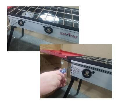
Remove all the screws that secure the front face plate.
