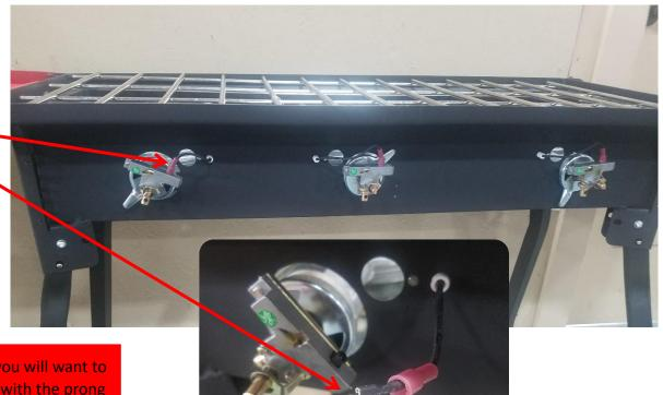
**Note:** After putting the stove back together, you will want to make sure the ignition knob is aligned correctly with the prong on the ignitor.
