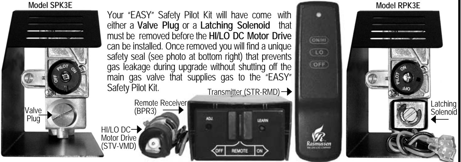
Your "EASY" Safety Pilot Kit will have come with either a **Valve Plug** or a **Latching Solenoid** that must be removed before the **HI/LO DC Motor Drive** can be installed. Once removed you will find a unique safety seal (see photo at bottom right) that prevents gas leakage during upgrade without shutting off the main gas valve that supplies gas to the "EASY" Safety Pilot Kit.
