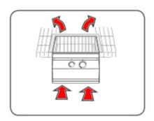
If installed under a patio roof, the cooking grid area should be fully covered by a chimney and exhaust hood. An exhaust fan with a rating of up to 1,000 CFM (472 liters per second) may be necessary to efficiently remove smoke and other Cooking byproducts from the covered area. Installation in fully enclosed patio areas is not recommended.
