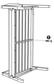
Once the component bolt is aligned and threaded, simply pull the guiding bolt from the end of the barrel nut.
