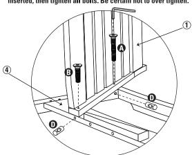
How to align barrel nuts and bolts.
