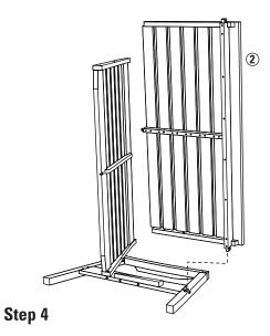
Using the provided allen wrench and guiding bolt  $\mathbf{G}$ , secure seat with barrel nut  $\mathbf{D}$  and SHORT bolt  $\mathbf{G}$  as shown.
