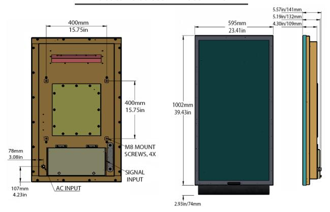
Speaker bar shown in bottom mount configuration can also be top mounted.
