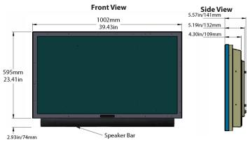
Speaker bar shown in bottom mount configuration can also be top mounted.
