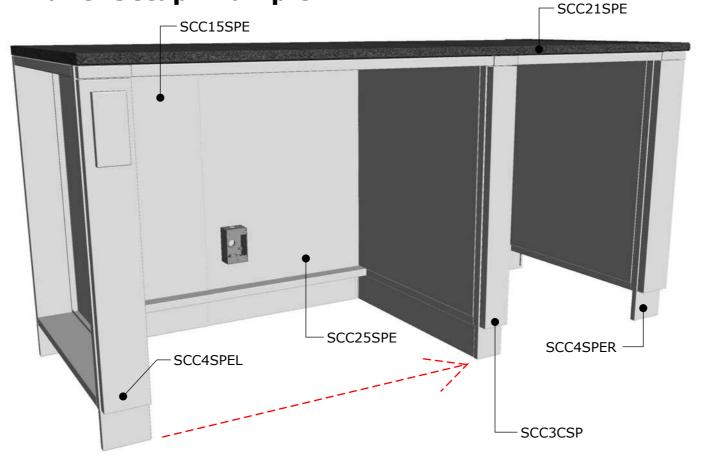
PLACE SPACER TO EXTEND APPLIANCE RUNS OR TO SEPERATE APPLIANCE TYPES
