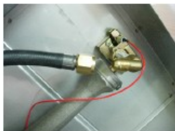
4.Connect Gas Hose with switch
