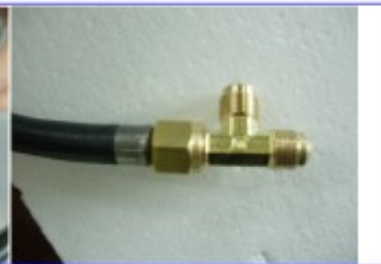
Attach one end of T-fitting to Regulator, the other end to Grill
