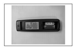
The receiver is powered by four 1.5V AA batteries located in a battery pack inside the heater component compartment. These batteries should be adequate for the heater operation for a whole season.
