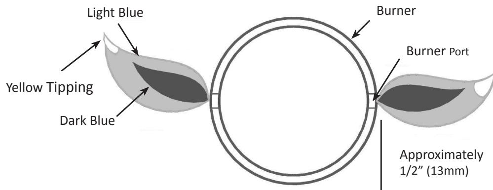
**Combustion Air Adjustment:** (This must be done by a qualified gas installer.) The air shutter is factory set and should not need adjusting under normal conditions. Under extreme field conditions, adjustments might be required. When the air shutter is adjusted correctly the flames will be dark blue, tipped with light blue and occasionally yellow.
