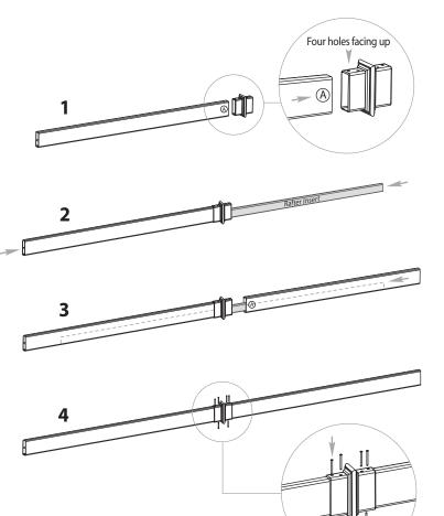
Pre-drill holes on bottom and top to accomodate for internal steel stiffener
