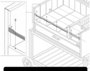
Fix the ember protector to the grill with the selft tapping screws. Drilling on grill body.
