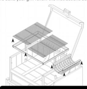
Remove Frame, fire box and grills to continue with DELTA assembly. The parts are not weld so, you just pull up to remove it.
