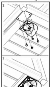
Position the rotating wheels by fastening them with the 5/8 "bolts to the base plate of the grill. If you have problems to fix any screws do not fix it. You will need at least 2 of them to fix the rotating wheels propietly.
