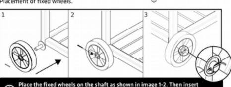
Place the fixed wheels on the shaft as shown in image 1-2. Then insert the lock in the shaft hole. Once the lock is in place, fold it as shown in figure 3, to ensure it remains properly attached.
