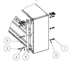
Attach the vent hood directly into the spacer through the mounting holes located on the rear hood cover plate. Fasten and tighten all hex nuts. Reference the parts list below to identify the hardware included with your wall mount spacer.
