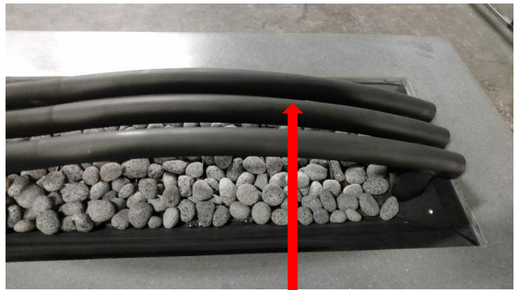
EXAMPLE OF POTENTIAL SOOT BUILDUP ON HEAT EXCHANGER TUBE
