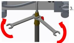
Tighten the fittings using two (2) wrenches. Failure to do so may result in fire.
