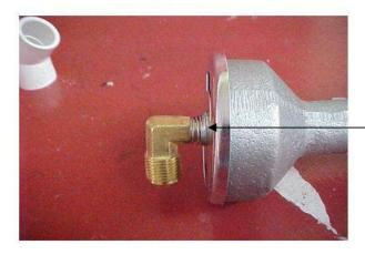
ALLOW SPRING TO KEEP ENOUGH PRESSURE ON THE PLATE SO THAT IT DOES NOT TURN FREELY BUT DO NOT OVER TIGHTEN.
