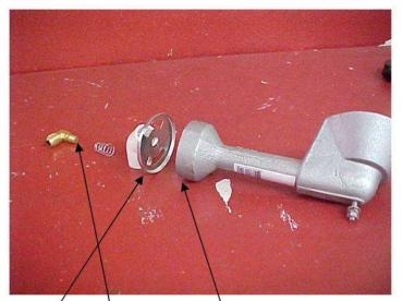
PUT SMALL JET END OF VALVE INTO SPRING. PUT PLATE ON BURNER AND SCREW JET END OF VALVE INTO FEMALE THREADS ON MAIN BURNER
