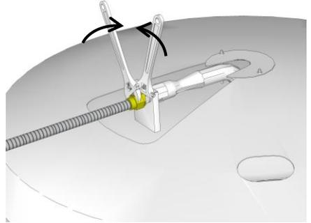
3. Attach flex line from the burner to gas valve as shown below.
