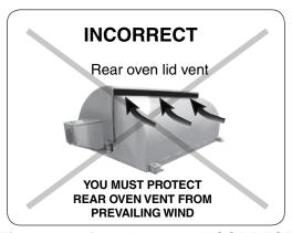
Fig. 10-3 Airflow direction - INCORRECT
