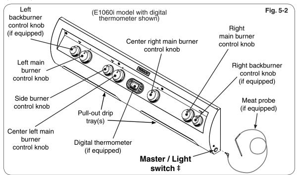
The master switch (Fig. 5-2) controls the power to all lights, igniters, and the thermometer. It allows the power to be turned on or off for safety and convenience. The switch will need to be turned on prior to each grill use, and turned off after each use.
