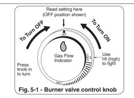
For your convenience and safety; when the control knob is turned to the ON position, the gas flow indicator will change from blue to red. (Red indicates gas flow.) See Fig. 5-1.
